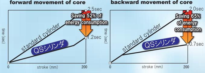
QS cylinder: bore of cylinder  $\Phi 200/\Phi 125$ , stroke 200mm standard cylinder: bore of cylinder  $\Phi$  200, stroke 200mm
