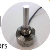
Cylinder attached with the sensors above monitors the amount of stroke for local squeezing. It removes shrinkage porosity.
